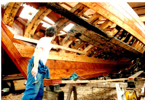
Pete Graham checking the run with a batten to see how the planks will land at the sternpost. He and Shaun White helped in the latter stages.
