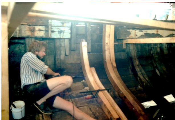
New framing replaced the old; drilling the frame off is Lawrence Weldon, who helped me in the earlier stages of the rebuild.
