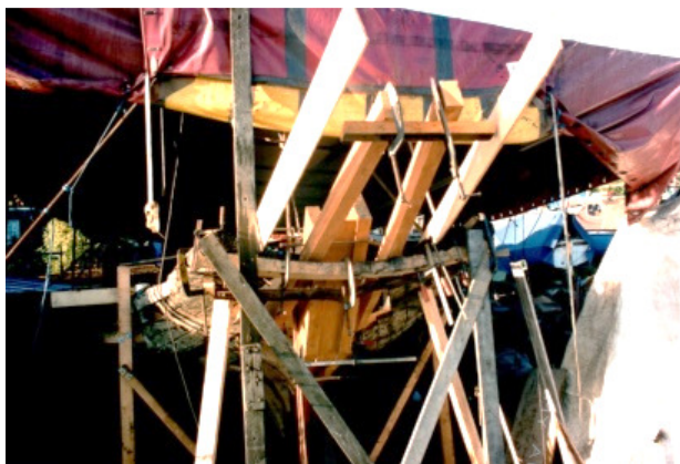
This view shows the new horn and quarter timbers going in to form the counter. This is always a delicate stage, as a fair sheer and pretty stern are crucial to the looks of the boat, but with no space to stand back and view the boat as a whole it is a fraught process.
