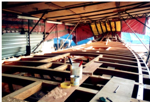
Here the deck structure nears completion. My Alice received a painted plywood deck, rather than the original laid one which can be seen in the earlier photo. This is strong and watertight, with few of the maintenance issues a traditional deck would entail.
